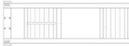
WP7 | WALL PANEL SUB-ASSEMBLY (x1) 1-7/16" x 28-1/16" x 89-1/2" (36 x 712 x 2274)
